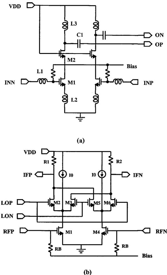
Fig. 2. (a) Simplified LNA schematic. (b) Simplified receive mixer schematic.
