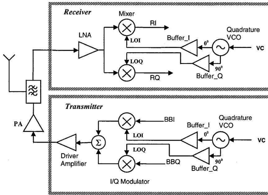
Fig. 1. Radio transceiver architecture.
