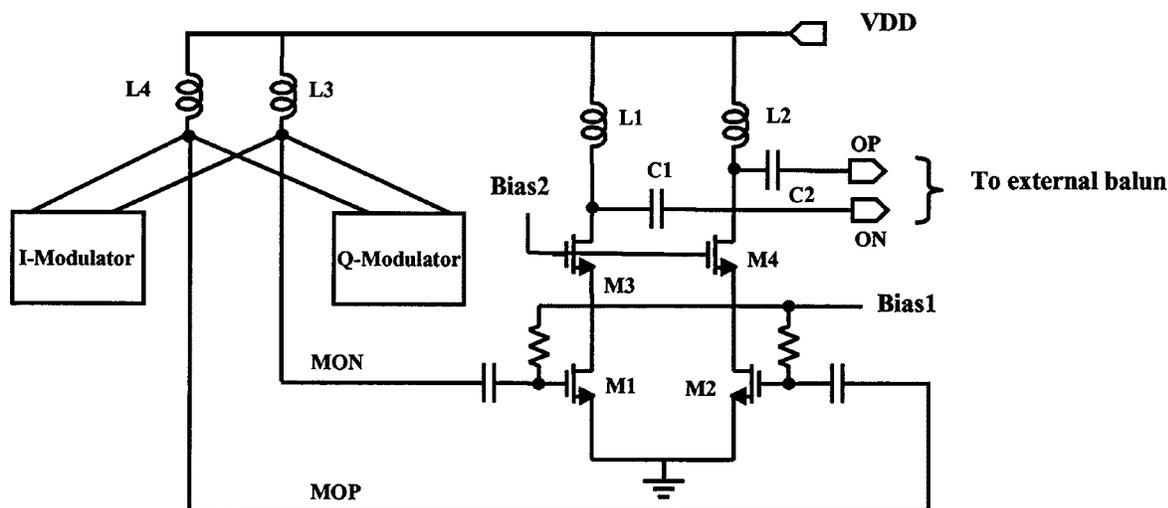
Fig. 4. Driver amplifier schematic.
