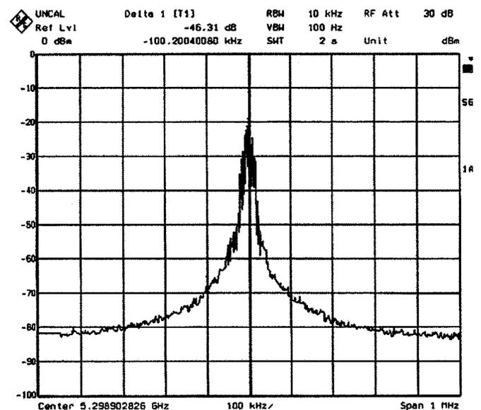
Fig. 8. Measured quadrature VCO phase noise.
