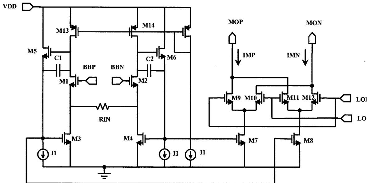
Fig. 3. Simplified modulator schematic.
