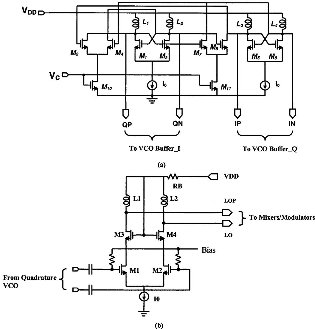
Fig. 5. (a) Quadrature VCO schematic. (b) VCO buffer schematic.
