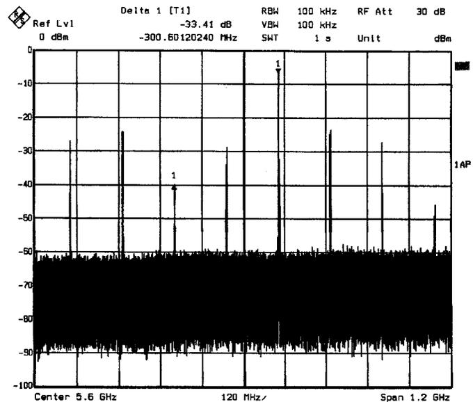
Fig. 10. Measured transmitter output spectrum.
